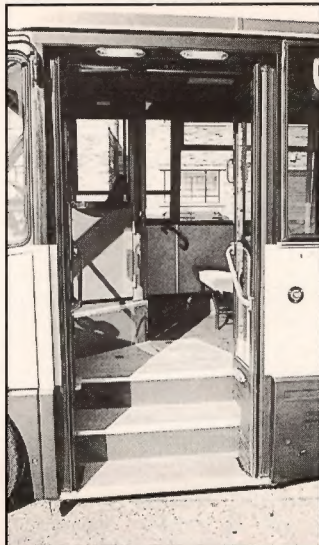
The DiPTAC 1997 Metrorider with a 250mm first step and all steps 300mm deep.
